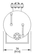
Exhaust outlet: 2" NPT Motive inlet: 2" NPT
