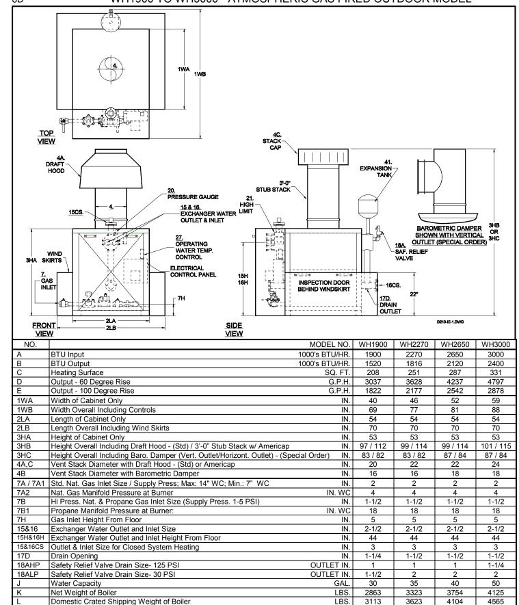
Recommended Clearances for Access: Inspection Doors 18"; Front (Cabinet Width 1WA + 10" For Exchanger Removal); Controls 24"; Electrical Panel 30"; Additional Space may be required by Local Codes
